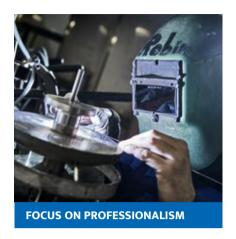
Our metal worker are certified according to the PED requirements and we have welding procedures for multiple stainless alloys.
